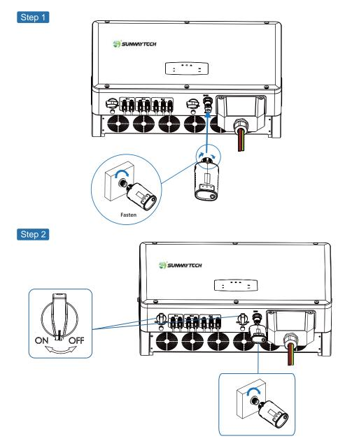
Turn on the DC switch and AC circuit breaker, and wait until the LED indicator on the monitoring module flashes, indicating that the monitoring module is successfully connected.
