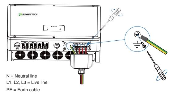
Unscrew the row of screws, insert the wire harness into the N, L1, L2, L3 caps one by one, and tighten the screws.
