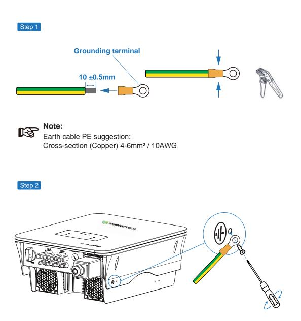
Grounding terminal is connected to the inverter at left or right side.
