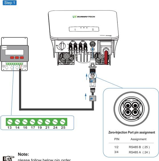
please follow below pin order RS485B (Pin 1/2) to three-phase meter (Pin 25) RS485A (Pin 3/4) to three-phase meter (Pin 24)
