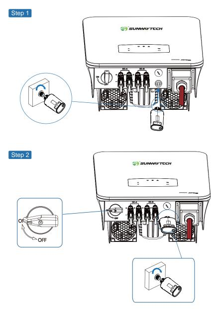
Turn on the DC switch and AC circuit breaker, and wait until the LED indicator on the monitoring module flashes, indicating that the monitoring module is successfully connected. **19** Electrical Connection
